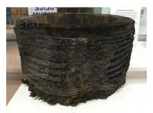
pipe and fitting them into couplers, such as this one pictured above, which seal due to the natural swelling of wet wood.
